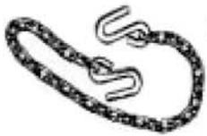
provisions for the connection of **safety chains**, which are required by most states. When connected, safety chains should have some slack to permit sharp turns but should not drag on the road. In addition, they should cross under the trailer tongue to help prevent the tongue from dropping to the road in the event the trailer separates from the tow vehicle.
