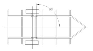
NOTE: When laying out the position for the axle(s), measuring from the front cross member should only be done if the cross member has been checked for squareness to the frame centerline. Any error in the cross member will be transferred to the axle and can result in poor tracking and excessive tire wear.
