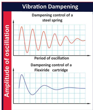
Rubber torsion axles offer a superior ride compared to leaf spring suspensions especially in unloaded trailers.
