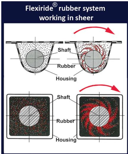
Flexiride® axles provide the smoothest ride in the market. The solid rubber cartridge works in shear as opposed to compression providing more angular compliance and superior vibration dampening compared to cord type axle systems. No shock absorbers are required due to rubber's natural vibration absorbing capabilities.
