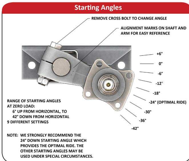
The splined joint connecting the spindle arm to the cartridge is exceptionally strong. Positioned at 6° increments, the splines provide a range of starting angles to fit a wide variety of applications and allowing trailer height adjustment. Unlike welded units, the Flexiride® spindle is easily replaced by removing the pinch bolt, nut and washer.
